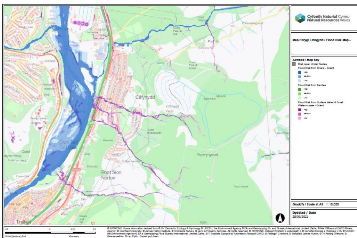
Figure 2: Natural Resources Wales' Flood Risk Assessment Wales (FRAW) map for rivers and ordinary watercourse and surface water flood risk at investigation area RCT10. Contains Natural Resources Wales information © Natural Resources Wales and database right. All rights reserved.
