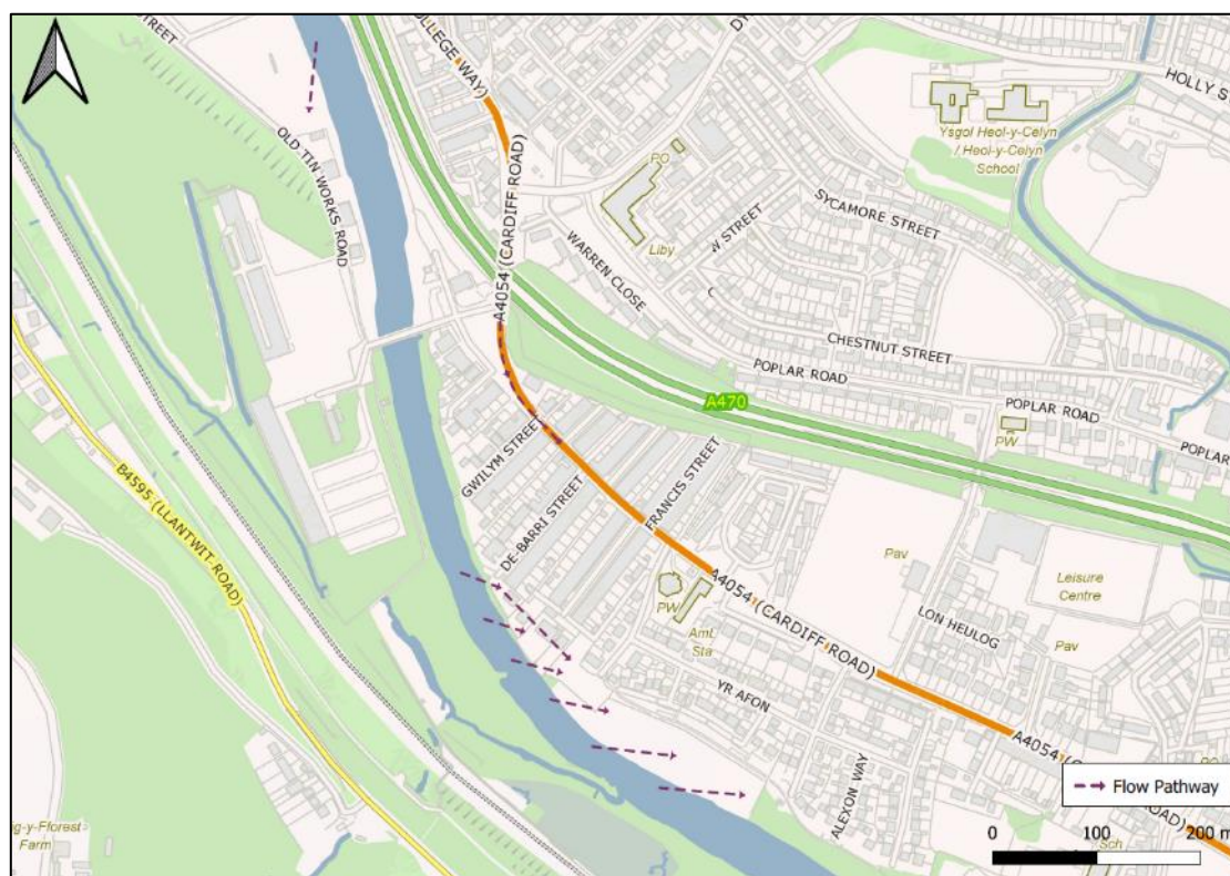
Figure 8: Flow pathways that caused flooding within Glyn-taf Rhydyfelin South
